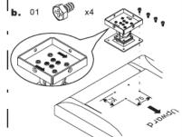
Secure bottom plate firmly to the wall with ,Make sure of direction correct during four expansion screws (not supplied). assembly. (as illustrated)
