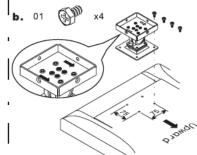
Secure bottom plate firmly to the wall with ,Make sure of direction correct during four expansion screws (not supplied). Assembly. (as illustrated)
