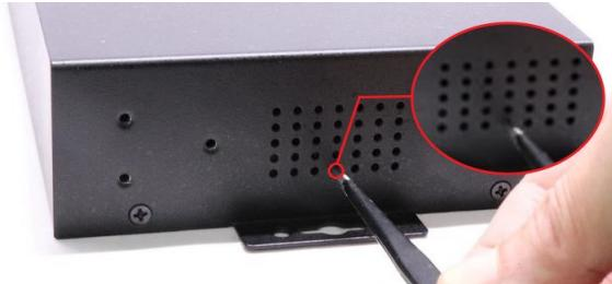
3. To do this, please use a paper clip or similar and press the button with not too much force and hold the button down while restoring power to the hub. After about 5-10 seconds you can release the reset button again..
