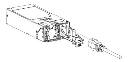
5. Secure the power cord by moving the buckle to the strain relief side of the power cord.
