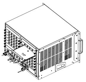
Install the VW884 video output board(s) to video output board slot(s).
