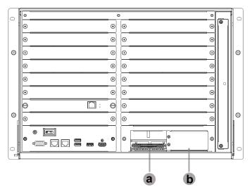
3. Slide the power module to the power slot. A click sound is made once the power module is properly installed.
