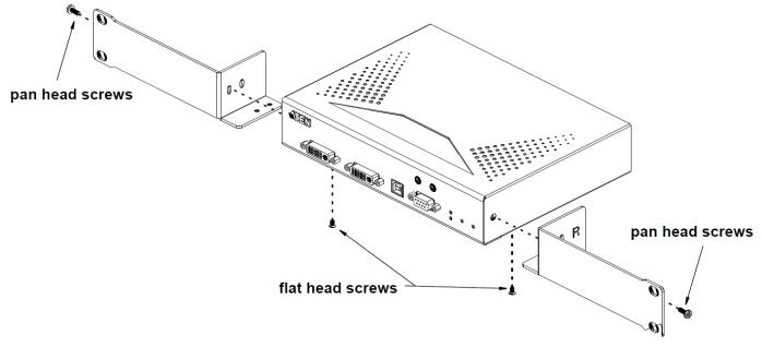
4. Screw the mounting brackets to the rack. The example used in the diagram below is a KE Series transmitter unit, the procedure for connecting to a receiver unit is identical.
